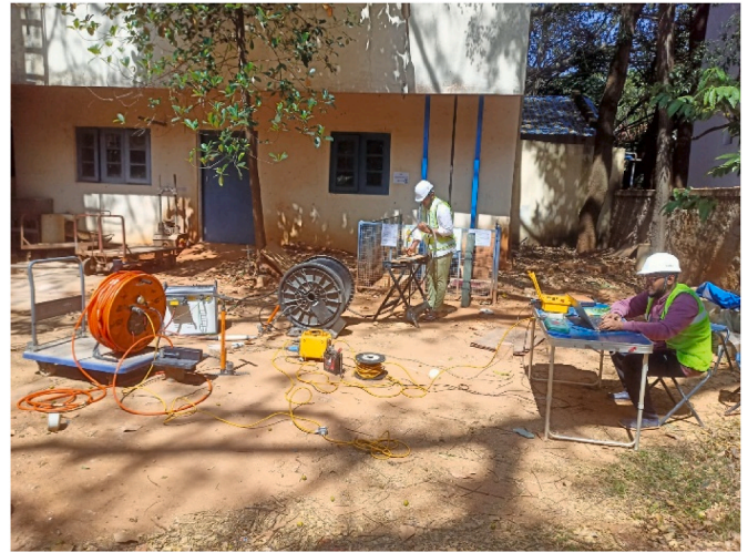
Fig. 9. Field setup for crosshole seismic testing at IISc, Bangalore.
